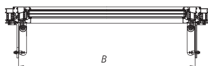
Fig. 20 B-B horizontal cross-section through mcr OSO THERM 75 smoke exhaust window in closed position
