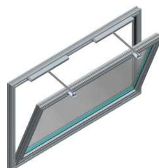
Fig. 54 mcr OSO THERM 75 smoke exhaust window with two HCV chain actuators
